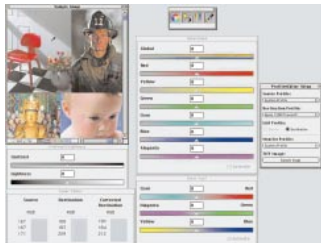
Figure 6. The tools and palettes available in Profile•Editor, and the supplied evaluation file for profile tuning and printing. Notice that the cursor is over the gray wall, and a set of RGB values is supplied in the Color Meter.
