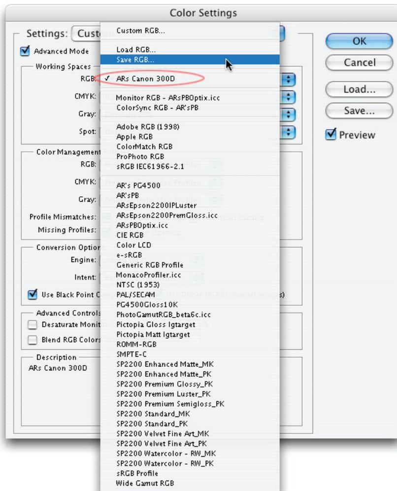
Figure 2. Save the settings of the ICC profile with a unique name.
