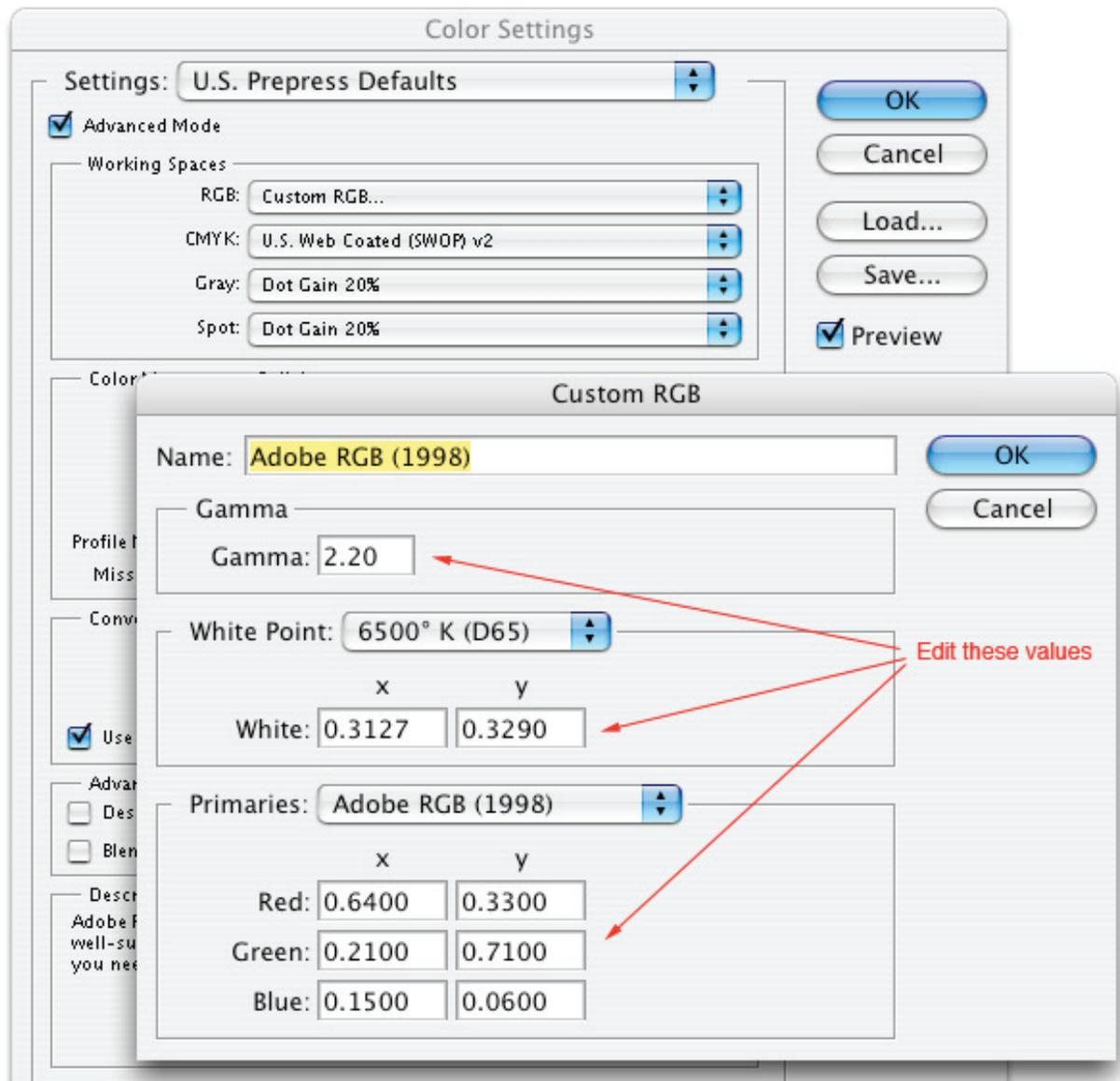
Figure 1. Alter the Working Space while looking at a preview of the camera file using the various fields above for best preview.
