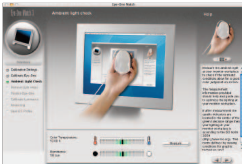
Figure 2: The main interface for Eye-One Match 3.0, where a user can measure the ambient light in the environment by the display system. The color temperature and luminance in LUX ++ is reported here.
